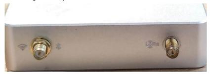
According to the silk-screen instructions on the antenna interface on the device side, install the Wi-Fi/BT antenna on the left and the LoRa antenna on the right as shown in the above figure.
